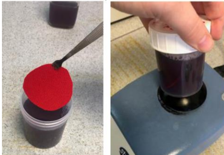
Test material is recovered in neutraliser and vortexed following 0 hour and 24 hour contact times, samples are enumerated following this step.
