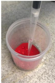
Test material inoculated (for 24 hour contact time samples are incubated following this step)
